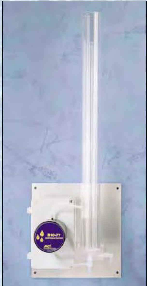
Particle sensor with flow control.
