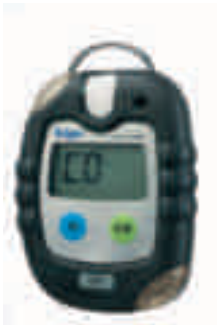
Dräger Pac 3000: Handy, reliable with large display.
