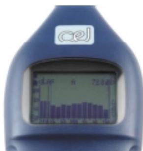
3 broadband plus 11 full octaves shown simultaneously on screen
