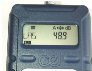
simple sound level meter display on CEL-320S instrument
